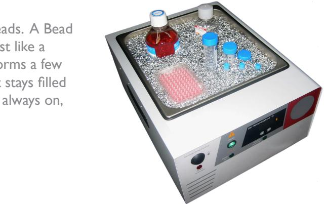
**BATH ARMOR™ BEADS.** Dry metallic beads that replace water in water baths, aluminum blocks in dry baths, ice in ice buckets, and give old equipment a cool, shiny, state-of-the-art upgrade.
